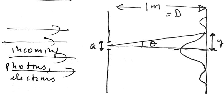
Any wave going through a narrow slit gives rise to a diffraction pattern, with the first minimum at angle  $\theta$  satisfying
