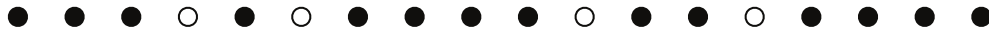
Figure 5.1: Partitioning N bosons into J possible states ( N = 14 and J = 5 shown). The N black dots represent bosons, while the J - 1 white dots represent markers separating the different single particle populations. Here n_1 = 3 , n_2 = 1 , n_3 = 4 , n_4 = 2 , and n_5 = 4 .
