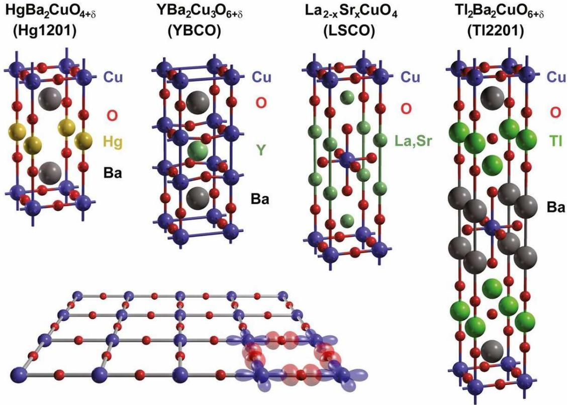
Figure 2.10: Unit cells of four high temperature cuprate superconductors. Lower left shows a sketch of the active electronic orbitals in the Cu-O planes. Image credit: N. Barišić *et al.*, *Proc. Nat. Acad. Sci.* **110**, 12235 (2013).
