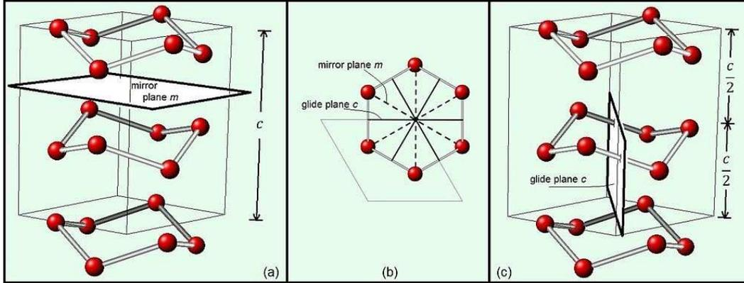
Figure 2.19: Structure of hexagonal  $\text{H}_2\text{O}$  ice, with red spheres showing location of oxygen atoms. The space group is  $P6_3/mmc$ . The  $6_3$  symbol indicates a sixfold screw axis. The first two  $m$  symbols indicate mirror planes perpendicular and parallel to the  $c$ -axis. The  $c$  symbol indicates a glide plane where the translation is along the  $c$ -axis. (Image credit: Wikipedia).
