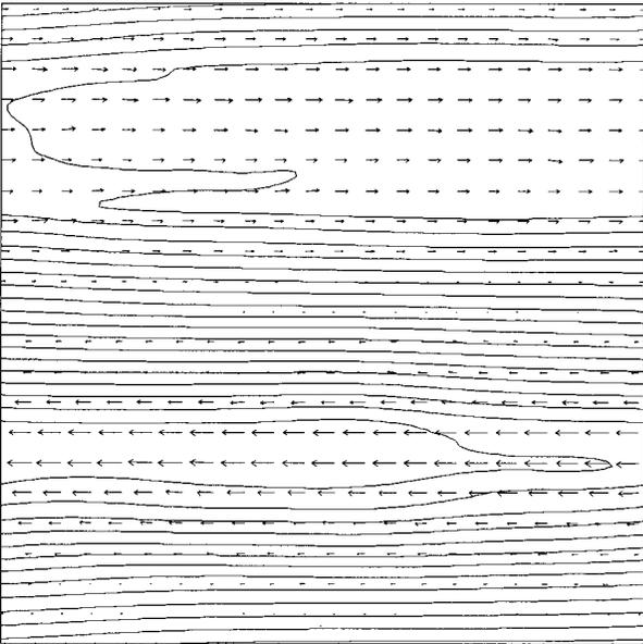
FIG. 20. Magnetic-field lines (solid curves) and velocity vectors (arrows) in a simulation of a uniform initial vertical field, viewed in  $(R, z)$  cross section. The axes are oriented as in Fig. 18. The flow evolves to two rapidly flowing channels. In cross section, they appear as oppositely moving radial streams. From Hawley and Balbus, 1992.
