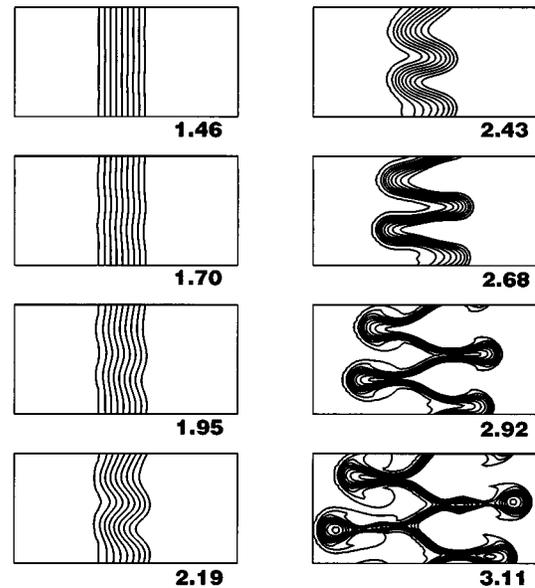
FIG. 18. Evolution of the vertical-field instability. The figure is an  $(R, z)$  cross section of field lines in an axisymmetric simulation of Keplerian differential rotation.  $R$  increases from left to right;  $z$  increases from bottom to top. The numbers give the time in orbits,  $2\pi/\Omega$ , where  $\Omega$  is the angular frequency at the center of the computational domain.
