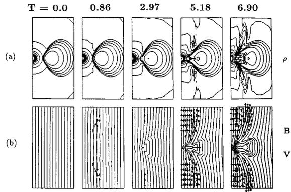
FIG. 22. Global evolution of an axisymmetric thick disk threaded by a uniform vertical field at time  $T=0$ , viewed in  $(R, z)$  cross section. The axes are oriented as in Fig. 18. The top row (a) shows the density; the bottom row (b) shows the magnetic-field lines (solid curves) and velocity vectors (arrows). The columns are labeled by orbital time. The weak-field instability leads promptly to rapid accretion. From Matsumoto *et al.*, 1996.
