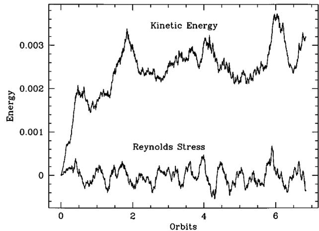
FIG. 12. Kinetic energy and Reynolds stress (in units normalized to the initial gas pressure) for an unstratified, adiabatic, Keplerian shearing box subject to external forcing. Gas is initially isothermal. Although the kinetic energy grows rapidly, the average Reynolds stress vanishes. The presence of turbulence does not necessarily lead to enhanced angular momentum transport in unmagnetized Keplerian disks.
