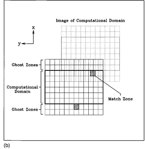
FIG. 7. Shearing box boundary conditions: (a) The computational domain is surrounded by identical domains moving with a fixed relative shear velocity; (b) Implementation of shearing box boundary conditions. The computational domain is surrounded by ghost zones corresponding to neighboring domains. Numerical values in these zones are obtained through interpolation of data from the corresponding matching zones.
