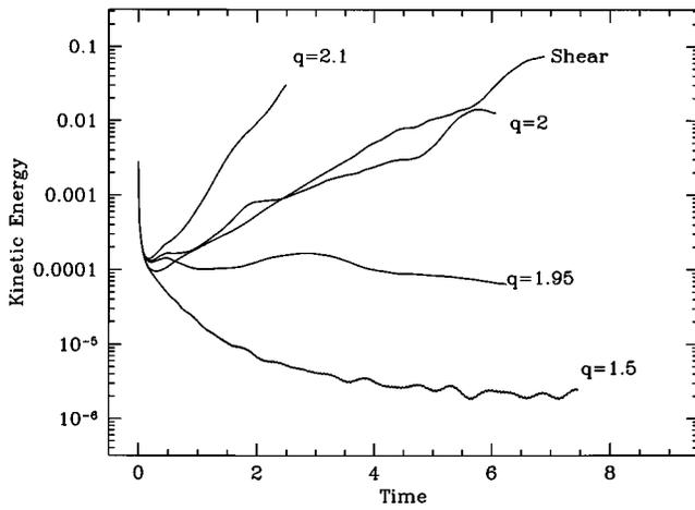
FIG. 9. Evolution of kinetic-energy fluctuations for different rotation profiles. The labels refer to the background angular velocity distribution, as given by  $\Omega(R) \sim R^{-q}$ . The curve labeled “Shear” has the same shear as the Keplerian  $q=1.5$  case, but without the dynamics of differential rotation (Coriolis force and tidal potential). The  $q=2$  curve corresponds to constant specific angular momentum,  $q=2.1$  to a Rayleigh-unstable profile.
