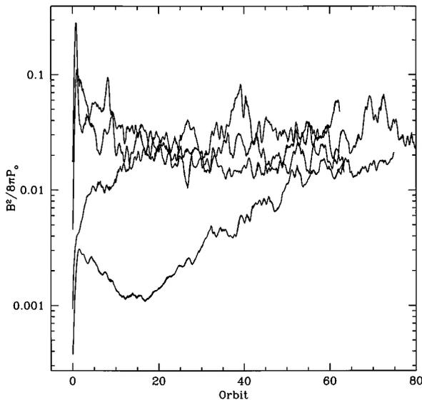
FIG. 23. Plots of normalized magnetic energy ( $\beta^{-1}$ ) as a function of time for a series of three-dimensional shearing box simulations. All simulations begin with a random magnetic field ( $\langle \mathbf{B} \rangle = 0$ ), but varying initial magnetic energy  $\langle B^2 \rangle$ . All initial conditions lead to turbulence with comparable magnetic energies. From Hawley *et al.*, 1996.
