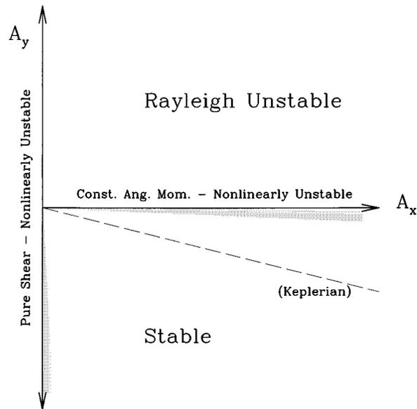
FIG. 13. Summary of hydrodynamic stability in the  $A_X$ - $A_Y$  plane. The  $A_X$  and  $A_Y$  axes correspond, respectively, to shear flow and constant specific-angular-momentum disk flow. Only points along the axes themselves were found to be nonlinearly unstable. (Numerical resolution uncertainty is represented by stippling near the axes.) Keplerian flow was found to be stable, well into any sensible nonlinear regime.
