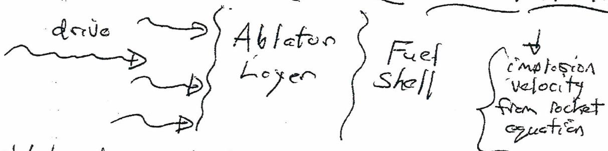
Oblator layer heats and expands thus compressing inner fuel layer (via PV work)
