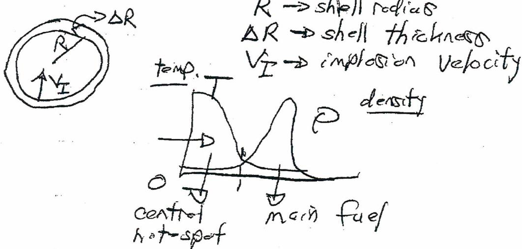
Idea is that burn initiates in central hot-spot, then propagates to main fuel shell.
