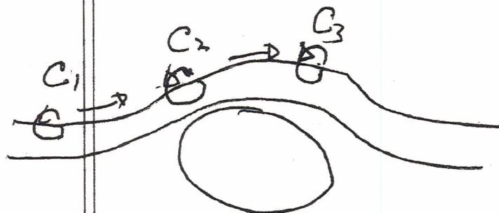
if  $\underline{\omega} = 0$  at any point along streamline, then Kelvin thm  $\Rightarrow \underline{\omega} = 0$  everywhere on streamline.
