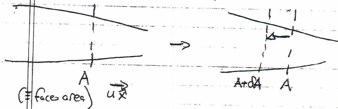
Net  $\frac{i}{\rho_0} = u \begin{bmatrix} A + \delta A & -A \end{bmatrix} = u \frac{\partial A}{\partial x} dx$
