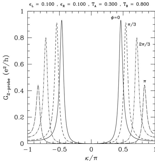
Figure 7.8: Two-probe conductance  $G(\phi, \kappa)$  of a model ring with two scatterers. The enclosed magnetic flux is  $\phi\hbar c/e$ , and  $\kappa = 2\pi kR$  (ring radius  $R$ ).  $G$  vs.  $\kappa$  curves for various values of  $\phi$  are shown.
