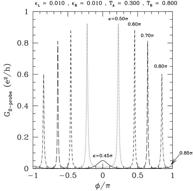
Figure 7.7: Two-probe conductance  $G(\phi, \kappa)$  of a model ring with two scatterers. The enclosed magnetic flux is  $\phi\hbar c/e$ , and  $\kappa = 2\pi kR$  (ring radius  $R$ ).  $G$  vs.  $\phi$  curves for various values of  $\kappa$  are shown. The coupling between leads and ring is one tenth as great as in fig. 7.6, and accordingly the resonances are much narrower. Note that the resonances at  $\kappa = 0.45\pi$  and  $\kappa = 0.85\pi$  are almost completely suppressed.
