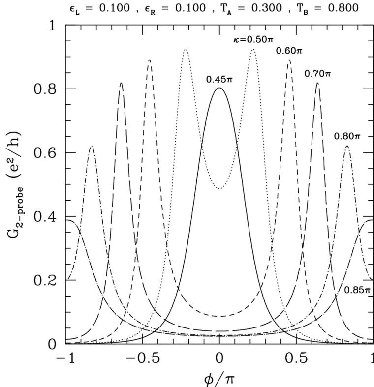
Figure 7.6: Two-probe conductance  $G(\phi, \kappa)$  of a model ring with two scatterers. The enclosed magnetic flux is  $\phi\hbar c/e$ , and  $\kappa = 2\pi kR$  (ring radius  $R$ ).  $G$  vs.  $\phi$  curves for various values of  $\kappa$  are shown.
