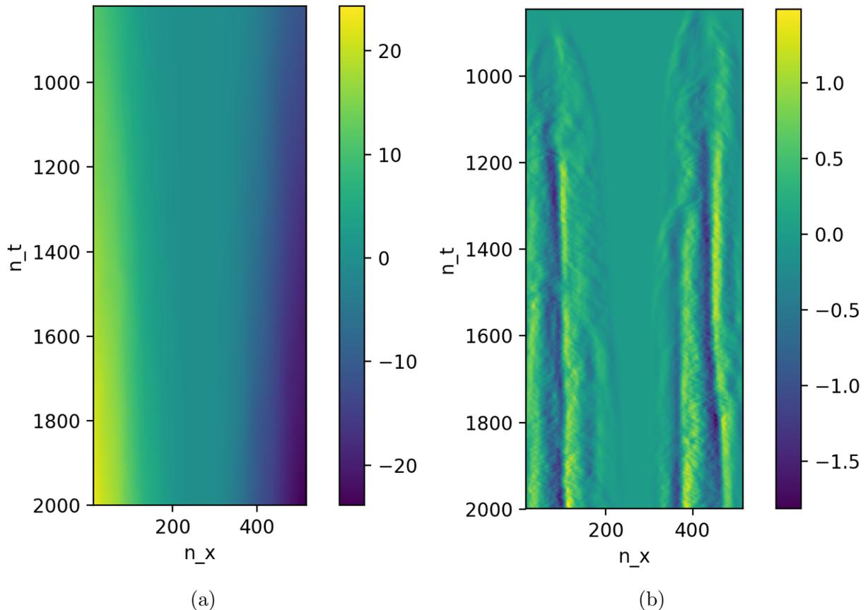
Figure 4: Plot showing mean density (a) and vorticity (b) evolution for  $f = 1$ . These snapshots show timesteps running from  $N_t \sim 8000$  to 2000 (vertical axis). The horizontal axis is position.
