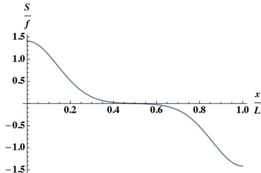
Figure 1: Plot of normalized source  $S(x)/f$  for the flux-driven simulations.
