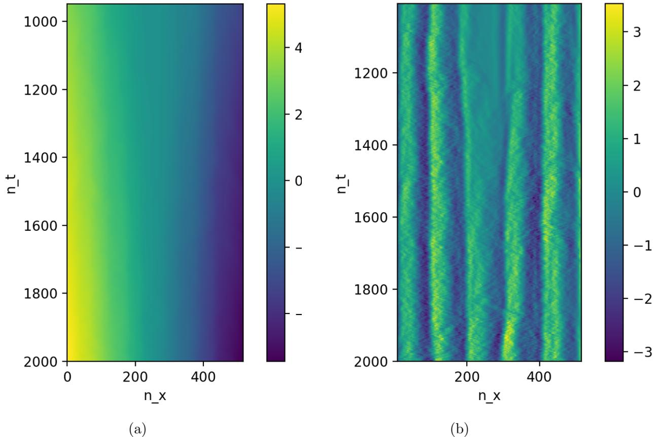
Figure 5: Plot showing mean density (a) and vorticity (b) evolution for  $f = 3$ . These snapshots show timesteps running from  $N_t \sim 1000$  to 2000 (vertical axis). The horizontal axis is position.
