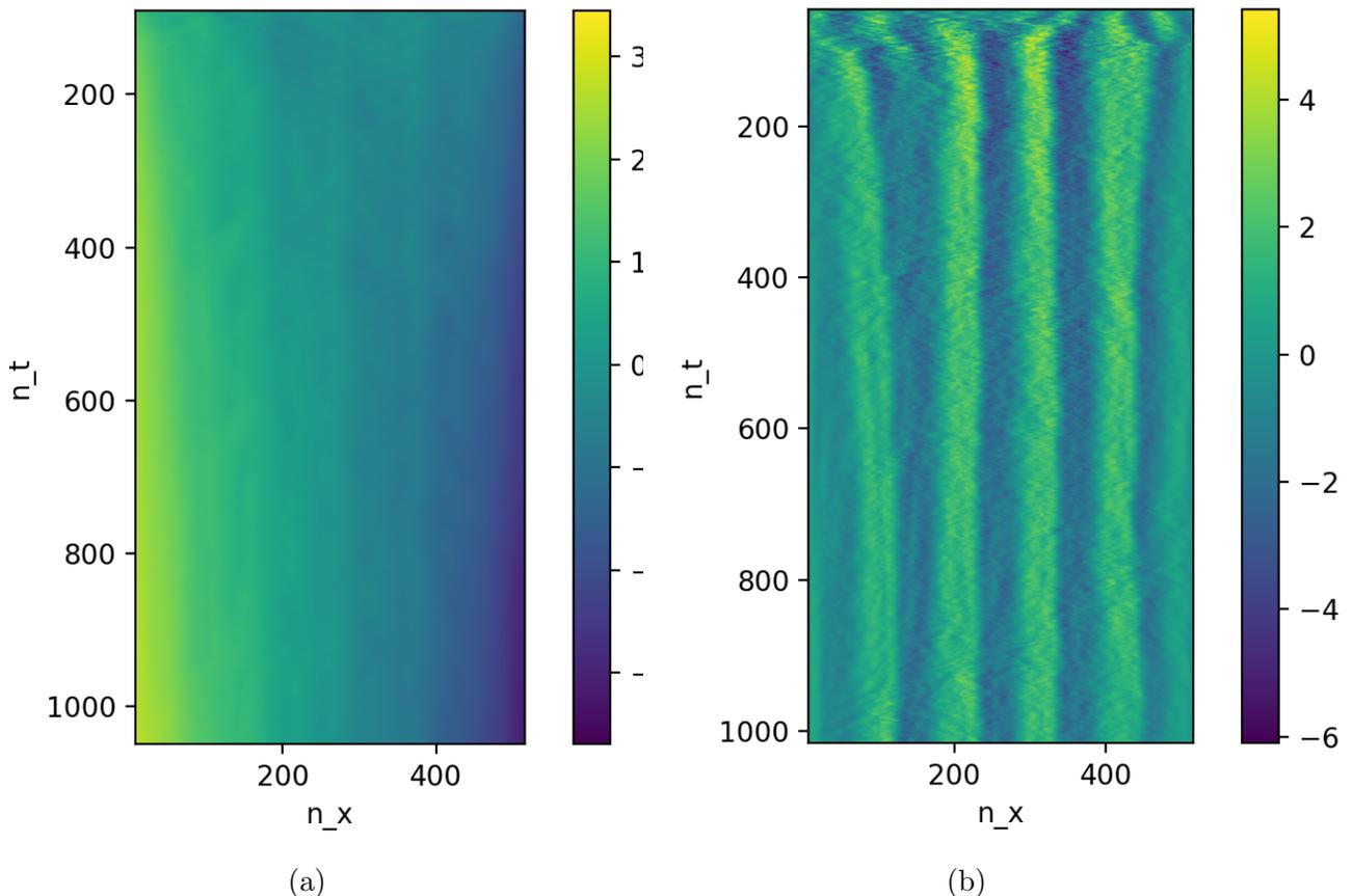
Figure 3: Plot showing mean density (a) and vorticity (b) evolution for  $\kappa = 3$ . These snapshots show timesteps running from  $N_t \sim 100$  to 1000 (vertical axis). The horizontal axis is position.
