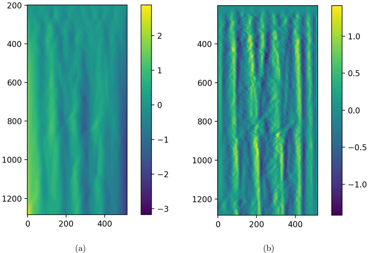
Figure 2: Plot showing mean density (a) and vorticity (b) evolution for  $\kappa = 1$ . These snapshots show timesteps running from  $N_t \sim 200$  to 1250 (vertical axis). The horizontal axis is position.
