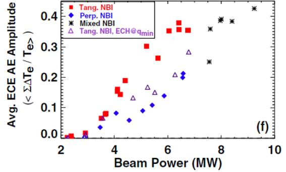
Figure 4: AE amplitudes measured by the ECE diagnostic show increasing amplitude with increasing injected beam power.<sup>2</sup> The different sets of points represent different injection geometries and heating combinations that affect AE activity. The threshold where AE activity increases is around  $P \approx 3$  MW.
