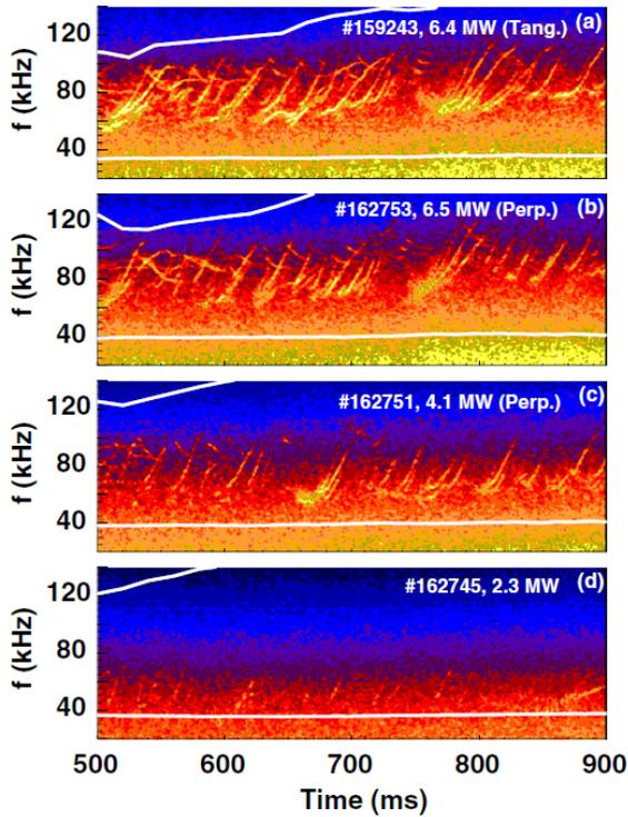
Figure 3: The CO<sub>2</sub> interferometer spectrogram shows little to no AE activity at lower beam powers and higher AE activity at higher beam powers.<sup>2</sup> Different injection geometries affect the amount of activity as shown in (a) and (b).
