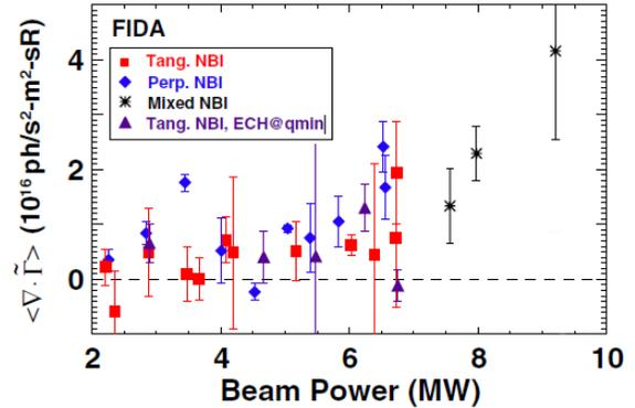
Figure 2: Calculated fast ion transport from the FIDA diagnostic show minimal transport at low beam power and a sudden increase in transport that seems to increase linearly with deviation from the critical gradient threshold located around  $P \approx 6\text{MW}$ .<sup>2</sup>
