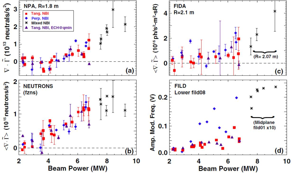
Figure 8: Transport measured by different fast ion diagnostics lead to different critical gradient thresholds due to the different sensitivities in phase space for each diagnostic<sup>2</sup>
