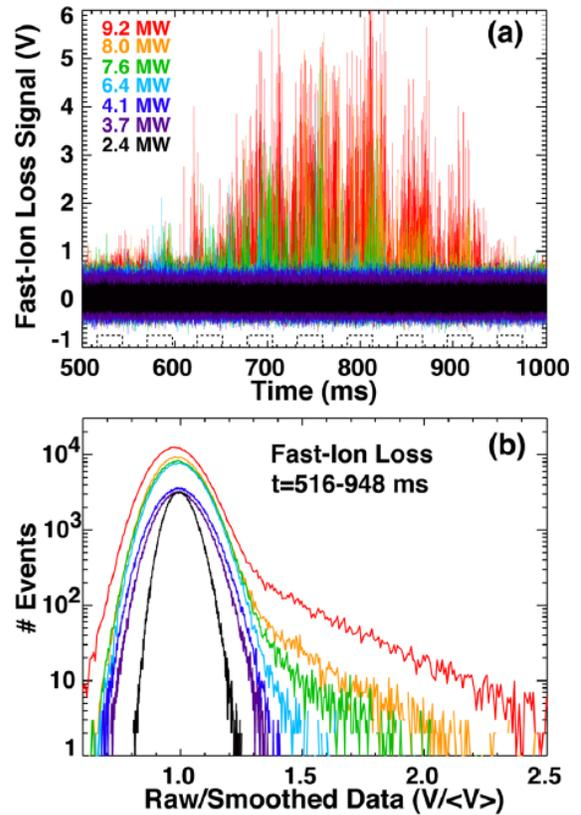
Figure 7: The FILD diagnostic measures increases in fast ion losses with increasing injected power in (a).<sup>1</sup> The distribution of the loss events (b) become more non-Gaussian and develops a fatter tail with increasing power.
