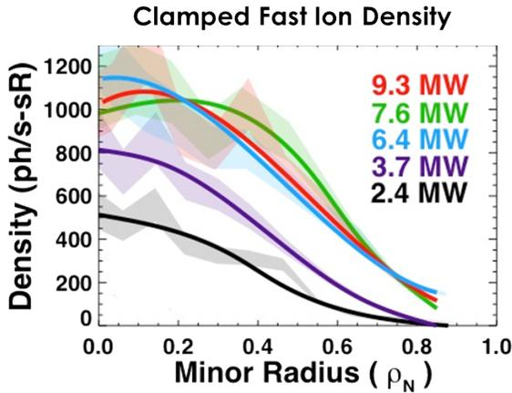
Figure 1: The FIDA diagnostic measures fast ion density in mostly co-passing orbits. Increase in beam power increases the density until the critical gradient threshold is reached. After that, the profile is resilient to further increases in the beam power.<sup>2</sup>
