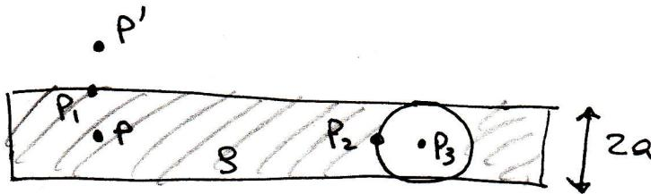
Electric field of slab:  $\sigma = S \cdot 2a$  is the charge per unit area
