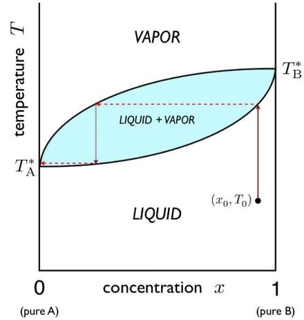
Figure 3: Phase diagram and distillation sequence for an ideal mixture.
