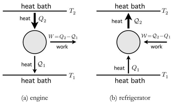
Figure 1: An engine (left) extracts heat  $Q_2$  from a reservoir at temperature  $T_2$  and deposits a smaller amount of heat  $Q_1$  into a reservoir at a lower temperature  $T_1$ , during each cycle. The difference  $W = Q_2 - Q_1$  is transformed into mechanical work. A refrigerator (right) performs the inverse process, drawing heat  $Q_1$  from a low temperature reservoir and depositing heat  $Q_2 = Q_1 + W$  into a high temperature reservoir, where  $W$  is the work done per cycle.
