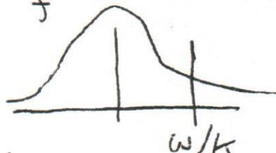
$\rightarrow$  Landau damping occurs due to wave particle resonance  $\omega/k \sim v$
