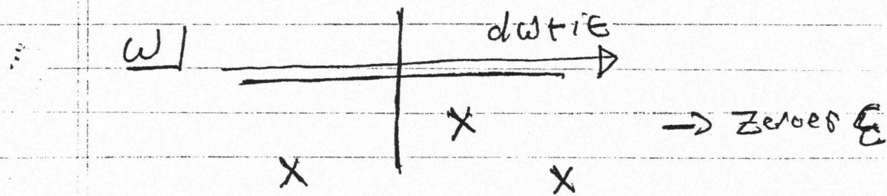
⇒ deform  $\omega$  contour downward till encircles zeroes.
