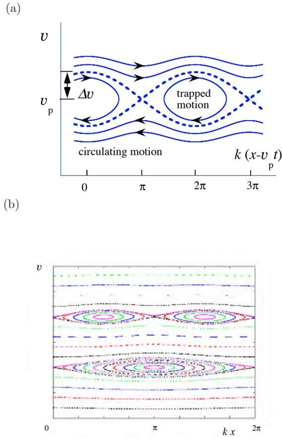
Fig. 3.5. (a) Structure of wave-particle resonance in phase space. The separatrix width is  $\Delta v \sim (q\phi_i/m)^{1/2}$ . Particles inside the separatrix (region of libration) undergo periodic motion on iso-energy contours and so are said to be trapped. Particles outside the separatrix circulate. (b) For several waves with distinct phase velocities, multiple resonance islands can co-exist and interact. [Courtesy of Prof. A. Fukuyama].
