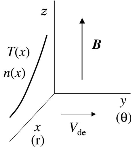
Fig. 3.14. Geometry of magnetized inhomogeneous plasma. The gradients and magnetic field are in the  $x$ -direction and  $z$ -direction, respectively. The electron diamagnetic drift velocity  $V_{de}$  is in the  $y$ -direction. Radial and poloidal directions  $(r, \theta)$  are also illustrated.
