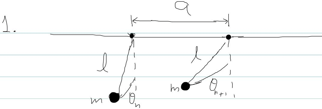
(i) **Dynamical variables:** There are many equivalent choices. The simplest one is the angular displacement of each mass,  $\theta_n$ , with respect to the equilibrium position (defined by all penduli masses directly below the wire and the wire being untwisted). We can be even more careful and define the sense of positive displacement, e.g., counter-clockwise when looking down the wire in the direction of increasing index "n". We won't need to be that specific.
