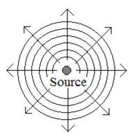
This diagram is a cross-section centered on the source. The circles show the locations of the wave peaks at a particular snapshot at time t; in fact, they are not circles but spherical surfaces, but they appear as circles in cross-section. The arrows show the direction of propagation of the wave at various points on the sphere.
