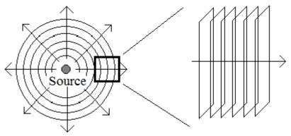
The planes on the right and the circles on the left once again represent the locations of maximum pressure, and the arrows show the direction of propagation of the wave.
