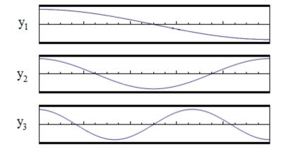
The frequency of the *n*th mode and the fundamental frequency are the same as for a pipe closed on both ends:
