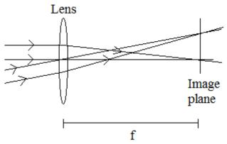
Rays coming in from infinity are focused at the focal point, where one can place the CCD or inspect the image with an eyepiece. Rays coming from different directions are focused to different points on the image plane; as you can see in the image above, the angle by which the points on the image plane are separated is the same as the angle by which the distant sources are separated.
