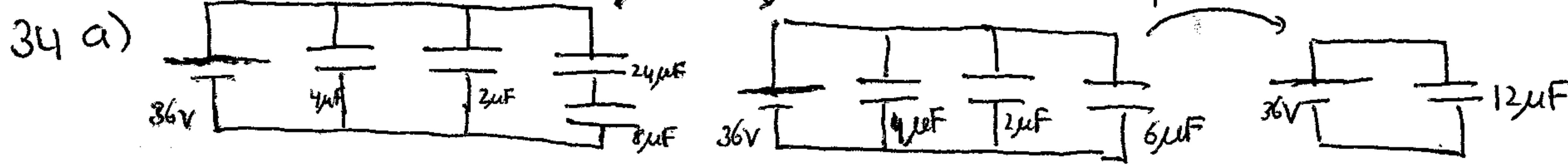
$$C_{eq} = 12 \mu F \text{ for this circuit.}$$
