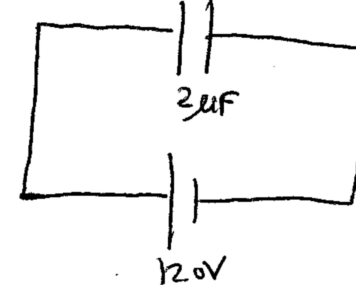
From the last picture  $C = \frac{Q}{\Delta V}$   $\Delta V = 12.0V$   $C = 2\mu F \Rightarrow Q = 2 \cdot 10^{-5} C$
