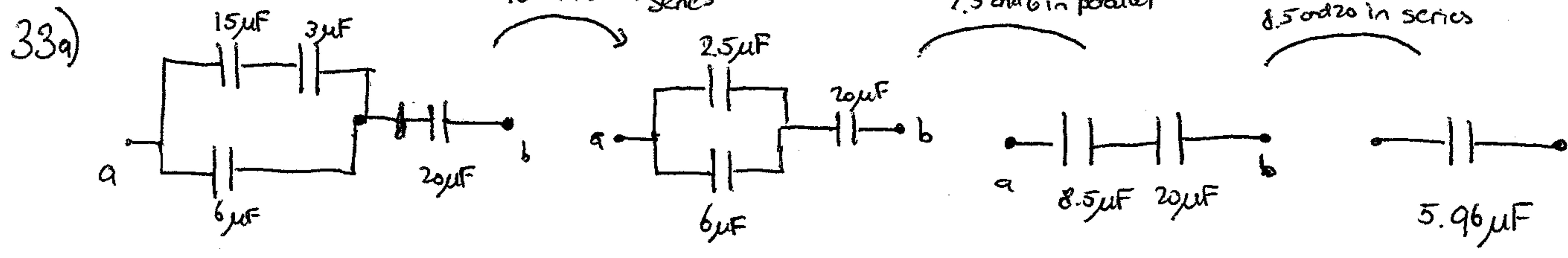
$$C_{eq} = 5.96 \mu F \text{ for this circuit}$$
