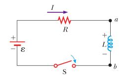
Given a 9-volt battery connected in series with a 3 mH inductor and a 0.5  $\Omega$  resistor. The switch is closed at t=0.
