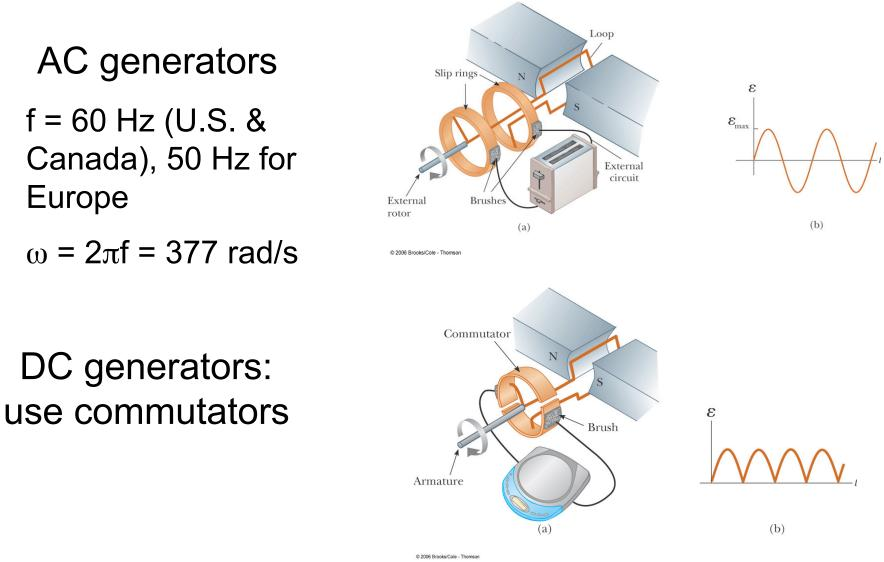
To get a DC output with minimal fluctuations: Use many loops & commutators distributed around the axis of rotation so that sinusoidal pulses overlap in phase
