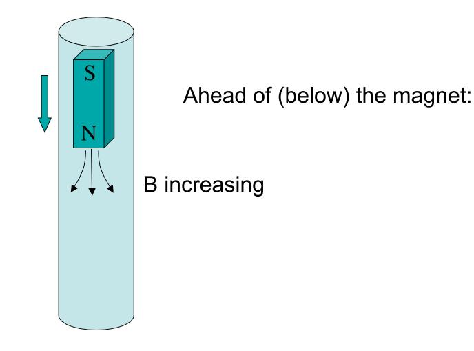
Drop a magnet down a cylindrical conductor, N-pole first. Currents are induced in the conductor to oppose the movement of the magnet:
