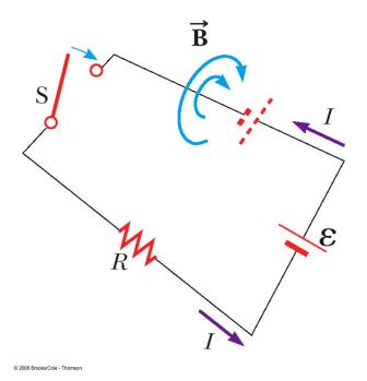
When switch is opened: current doesn't immediately fall to zero.
