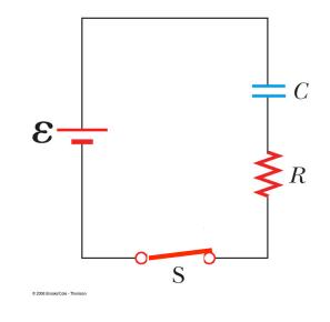
Immediately after time t=0: Current starts to flow. Charge starts to accumulate on Capacitor (at a rate I=dQ/dt).
