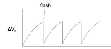
Solution: Have the flash point be equal to 0.63  $\Delta V_{C,max}$
