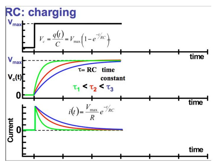
You want to make a so-called flasher circuit that charges a capacitor through a resistor up to a voltage at which a neon bulb discharges once every 5.0 sec. If you have a 10 microfarad capacitor what resistor do you need?
