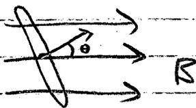
$\text{Flux} = \Phi_B = BA \cos 30^\circ = \boxed{0.866 \times 10^{-7} \text{ Tm}^2}$
