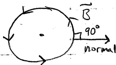
$\Phi_B = BA \cos \theta$ , but  $\theta = 90^\circ$  because the B field curls around and the normal to the surface is radially outward.  $\boxed{\text{Flux} = 0}$
