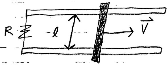
When you move the bar the area will change, so the flux will change, so there will be an induced voltage and therefore an induced current.
