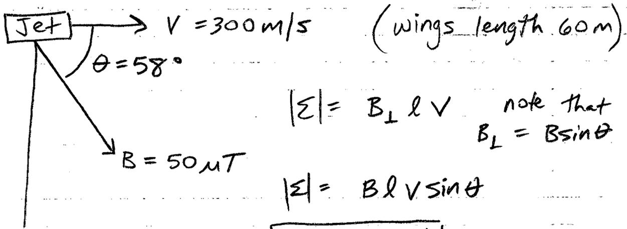
$|\mathcal{E}| = B_{\perp} l v$  note that  $B_{\perp} = B \sin \theta$
