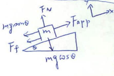
F<sub>f</sub> is the friction,  $F_f = F_N \cdot \mu = mg \cos \theta \cdot \mu$ Along x direction:  $\sum F_x = 0$
