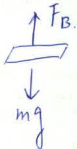
$$\text{Buoyancy } F_B = V_{\text{in}} f_{\text{water}} g. \quad V_{\text{in}} = 0.6 V.$$
