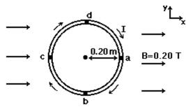
The magnitude of the magnetic moment of the loop is 0.75 A • m<sup>2</sup>. A uniform external magnetic field, B = 0.20 T in the positive x-direction, is present. The loop is released from rest. The initial motion of the loop is described by:
