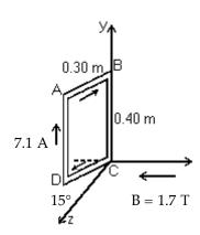
A rigid rectangular loop, which measures 0.30 m by 0.40 m, carries a current of 7.1 A, as shown. A uniform external magnetic field of magnitude 1.7 T in the negative x-direction is present. Segment CD is in the x-z plane and forms a  $15^{\circ}$  angle with the z-axis, as shown. The y-component of the magnetic force on segment AB is closest to:
