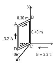
A rigid rectangular loop, which measures 0.30 m by 0.40 m, carries a current of 3.2 A, as shown. A uniform external magnetic field of magnitude 2.2 T in the negative x-direction is present. Segment CD is in the x-z plane and forms a  $36^{\circ}$  angle with the z-axis, as shown. The y-component of the magnetic force on segment AB is closest to:
