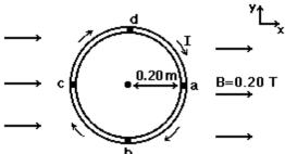
The magnitude of the magnetic moment of the loop is  $0.75 \text{ A} \cdot \text{m}^2$ . A uniform external magnetic field, B = 0.20 T in the positive x-direction, is present. The loop is released from rest. The initial motion of the loop is described by:
