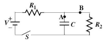
A long time after the switch is closed the current at the point labeled "A" is
