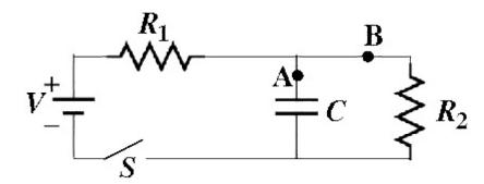
Long after the switch is closed the potential difference between the negative terminal of the battery and the wire at the point labeled "A" is
