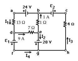
It is not necessary to solve the entire circuit. The current I<sub>1</sub> is closest to:
