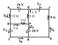
It is not necessary to solve the entire circuit. The current I2 is closest to:
