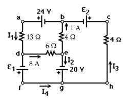
It is not necessary to solve the entire circuit. The current  $I_1$  is closest to:
