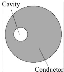
If a positive charge is placed on the conductor, the electric field in the cavity
