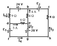
It is not necessary to solve the entire circuit. The current I2 is closest to: A) -1 A B) 9 A C) 1 A D) zero E) -9 A
