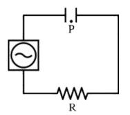
The plates of the capacitor are disks with a radius R. The plates are separated by a distance d. Directly between the two plates (a distance d/2 from each plate), a distance R/2 from the center axis, is location P. At location P,
