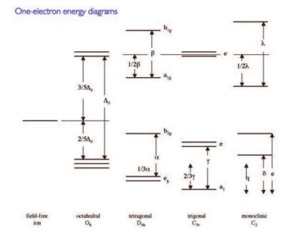
Figure 14.4: The splitting of one-electron states in different crystal field environments.
