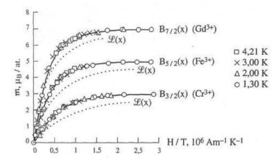
Figure 14.5: Reduced magnetization curves for three paramagnetic salts and comparison with Brillouin theory predictions.  $\mathcal{L}(x) = B_{J\to\infty}(x) = \operatorname{ctnh}(x) - x^{-1}$  is the Langevin function.
