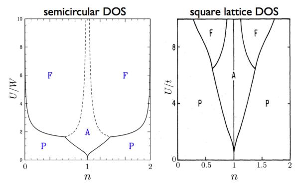
Figure 14.7: Mean field phase diagram of the Hubbard model, including paramagnetic (P), ferromagnetic (F), and antiferromagnetic (A) phases. Left panel: results using a semicircular density of states function of half-bandwidth *W*. Right panel: results using a two-dimensional square lattice density of states with nearest neighbor hopping *t*, from J. E. Hirsch, *Phys. Rev. B* **31**, 4403 (1985). The phase boundary between F and A phases is first order.
