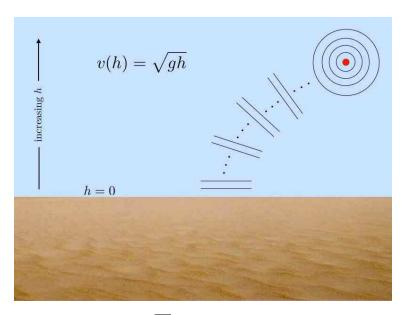
Figure 5.5: For shallow water waves,  $v = \sqrt{gh}$ . To minimize the propagation time from a source to the shore, the waves break parallel to the shoreline.
