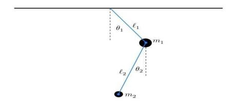
Figure 6.3: The double pendulum, with generalized coordinates  $\theta_1$  and  $\theta_2$ . All motion is confined to a single plane.
