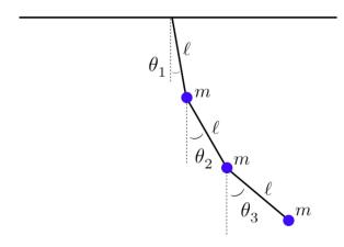
Figure 10.5: The triple pendulum.
