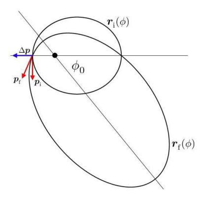
Figure 9.8: At perigee of an elliptical orbit  $r_i(\phi)$ , a radial impulse  $\Delta p$  is applied. The shape of the resulting orbit  $r_f(\phi)$  is shown.
