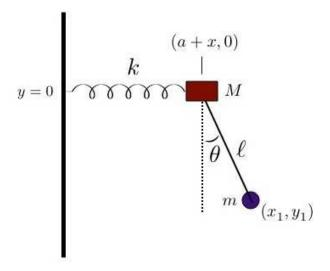
Figure 6.2: The spring–pendulum system.
