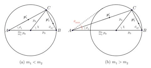
Figure 11.3: Scattering when particle 2 is initially at rest.
