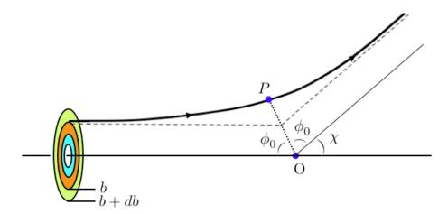
Figure 11.6: Scattering in the CM frame. O is the force center and P is the point of periapsis. The impact parameter is b, and  $\chi$  is the scattering angle.  $\phi_0$  is the angle through which the relative coordinate moves between periapsis and infinity.
