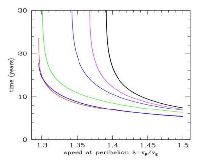
Figure 9.12: Total time for Earth-Neptune mission as a function of dimensionless velocity at perihelion,  $\lambda = v_{\rm p}/v_{\rm E}$ . Six different values of  $\kappa$ , the value of perijove in units of the Jovian radius, are shown:  $\kappa = 1.0$  (thick blue),  $\kappa = 5.0$  (red),  $\kappa = 20$  (green),  $\kappa = 50$  (blue),  $\kappa = 100$  (magenta), and  $\kappa = \infty$  (thick black).
