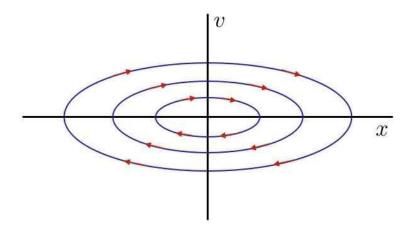
Figure 3.3: Phase curves for the harmonic oscillator.
