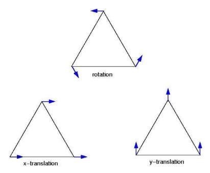
Figure 10.7: Zero modes of the mass-spring triangle.
