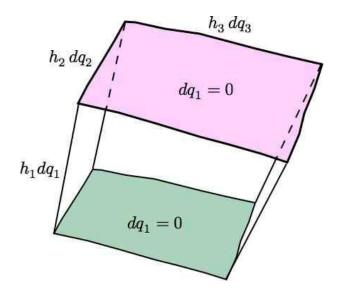
Figure 2.2: Volume element  $\Omega$  for computing divergences.
