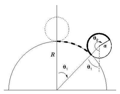
Figure 8.1: A cylinder of radius a rolls along a half-cylinder of radius R. When there is no slippage, the angles  $\theta_1$  and  $\theta_2$  obey the constraint equation  $R\theta_1 = a(\theta_2 - \theta_1)$ .
