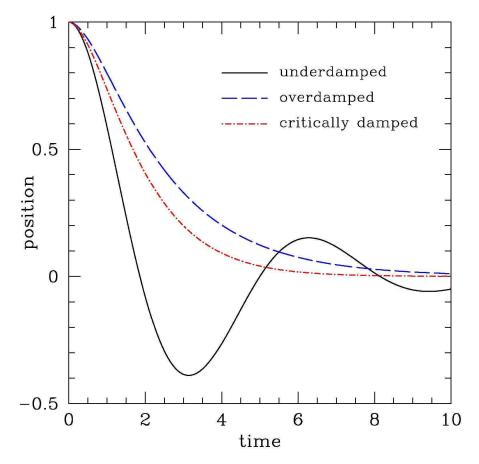
Figure 4.1: Three classifications of damped harmonic motion. The initial conditions are x(0) = 1,  $\dot{x}(0) = 0$ .
