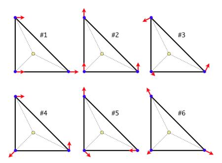
Figure 10.4: Normal modes of the 45° right triangle. The yellow circle is the location of the CM of the triangle.
