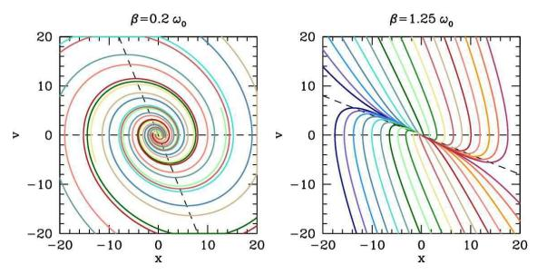
Figure 4.2: Phase curves for the damped harmonic oscillator. Left panel: underdamped motion. Right panel: overdamped motion. Note the *nullclines* along v=0 and  $v=-(\omega_0^2/2\beta)x$ , which are shown as dashed lines.
