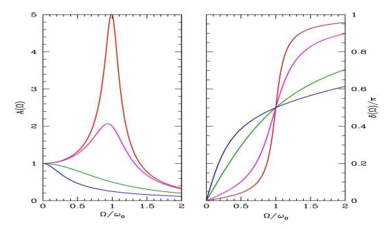
Figure 4.3: Amplitude and phase shift *versus* oscillator frequency (units of  $\omega_0$ ) for  $\beta/\omega_0$  values of 0.1 (red), 0.25 (magenta), 1.0 (green), and 2.0 (blue).
