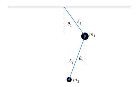
Figure 10.2: The double pendulum.
