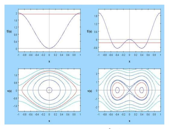
Figure 7.2: The effective potential  $U_{\rm eff}(\theta) = mga \left[1 - \cos\theta - \frac{\omega^2}{2\omega_0^2} \sin^2\theta\right]$ . (The dimensionless potential  $\tilde{U}_{\rm eff}(x) = U_{\rm eff}/mga$  is shown, where  $x = \theta/\pi$ .) Left panels:  $\omega = \frac{1}{2}\sqrt{3}\,\omega_0$ . Right panels:  $\omega = \sqrt{3}\,\omega_0$ .
