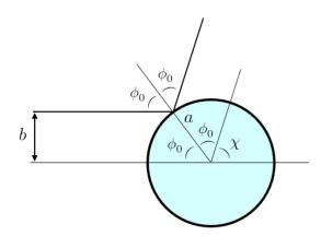
Figure 11.7: Geometry of hard sphere scattering.
