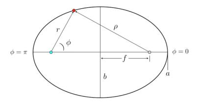
Figure 9.6: The Keplerian ellipse, with the force center at the left focus. The focal distance is  $f = \varepsilon a$ , where a is the semimajor axis length. The length of the semiminor axis is  $b = \sqrt{1 - \varepsilon^2} a$ .
