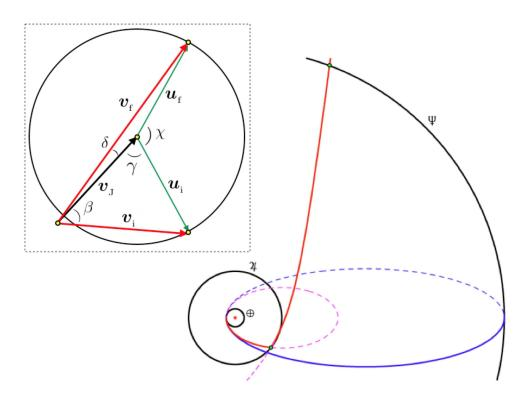
Figure 9.11: Mission to Neptune. The figure at the lower right shows the orbits of Earth, Jupiter, and Neptune in black. The cheapest (in terms of energy) direct flight to Neptune, shown in blue, would take 30.6 years. By swinging past the planet Jupiter, the satellite can pick up great speed and with even less energy the mission time can be cut to 8.5 years (red curve). The inset in the upper left shows the scattering event with Jupiter.
