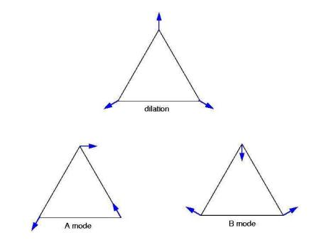
Figure 10.8: Finite oscillation frequency modes of the mass-spring triangle.
