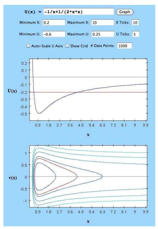
Figure 3.5: Phase curves for the Kepler effective potential  $U(x) = -x^{-1} + \frac{1}{2}x^{-2}$ .
