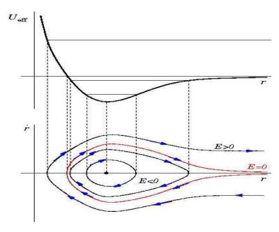
Figure 9.4: The effective potential for the Kepler problem, and associated phase curves. The orbits are geometrically described as conic sections: hyperbolae (E > 0), parabolae (E = 0), ellipses  $(E_{\min} < E < 0)$ , and circles  $(E = E_{\min})$ .
