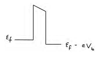
Show that if the voltage bias is greater than the work function, the electron in effect needs to tunnel through a triangular barrier. What is the 'effective width' of the barrier that the electron sees?
