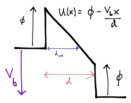
When  $V_b \ge \phi$ , the height of the barrier becomes zero at some smaller distance  $d_{eff} \le d$ and the electron effectively sees a triangular barrier. The effective width is where  $\phi - V_b x/d = 0$  or  $x = \phi d/V_b$ .
