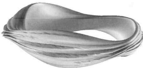
FIGURE 19 Development of a ballooning-kink mode in a torus. Note how a side view of the finger formation reveals the tendency of the ballooning mode to crenelate the plasma and break it into ribbons. Courtesy of S. C. Jardin and the Center for Extended MHD Modeling, Princeton Plasma Physics Laboratory.
