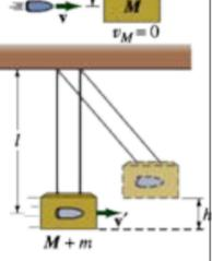
Can measure bullet speed by watching how much block rises after impact!
