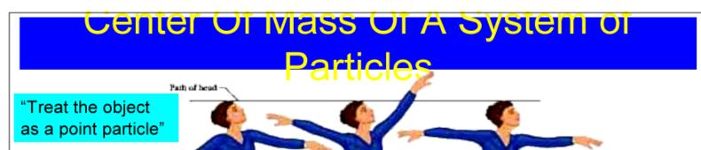
Center of Mass (cm) of a system of particles is the point that moves as though (1) all of system's mass was concentrated there (2) all external forces were applied there
