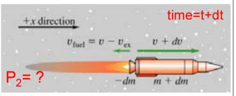
In time dt, rocket ejects burnt mass -dm with rel. velocity v<sub>ex</sub>
