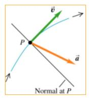
When particle travels along curved path with decreasing speed,  $\vec{a}$  has components  $\perp \&$  anti- $\parallel$  to  $\vec{v}$  & points behind the *normal* to the path
