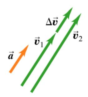
When  $\vec{a} \parallel \vec{v}$  or anti- $\parallel$ vector addition  $\Rightarrow$ change in magnitude of  $\vec{v}$ but not its direction
