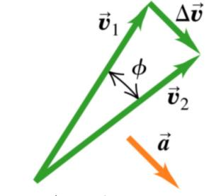
When  $\vec{a} \perp \vec{v}$ vector addition  $\Rightarrow$ change the direction of  $\vec{v}$ but not its magnitude (speed remains unchanged!)
