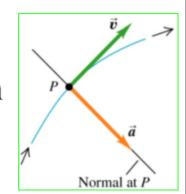
When particle travels along curved path with increasing speed,  $\vec{a}$  has components  $\perp \& \parallel$  to  $\vec{v}$  & points ahead of the *normal* to the path
