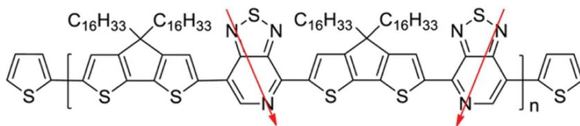
**Scheme 1.** Molecular structure and regioregularity pattern of PCDTPT. The arrows are guides to the eye to highlight stereoregularity.
