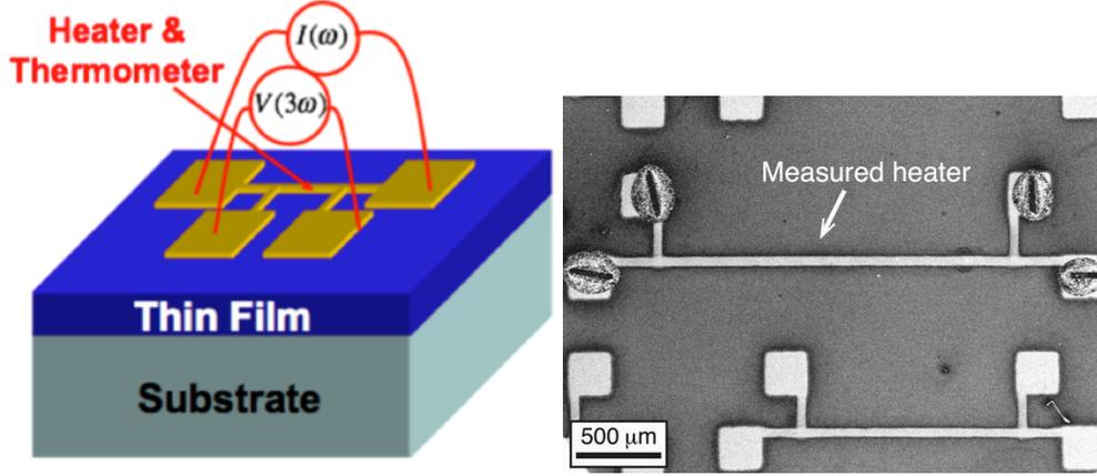
Fig. 1 Schematic diagram (left) and (a scanning electron microscopic (SEM) image (right) of a device for  $3\omega$  measurement for thin film sample [refers 3 and 4].
