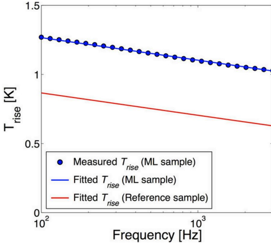
Fig. 3 Experimental temperature rise with fitting results as a function of frequency measured by  $3\omega$  method [refer 4].
