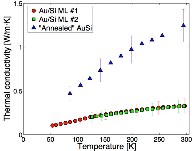
Fig. 4 Measured thermal conductivity as a function of temperature, where the measurement was conducted in vacuum chamber. Samples before (circle) and after (triangle) annealing process was compared [refer 4].
