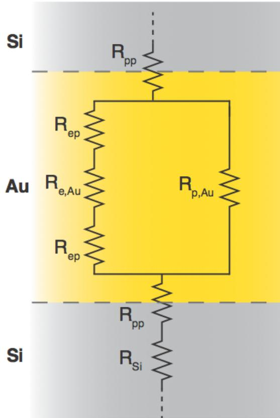
Fig. 2 Schematic of equivalent circuit of thermal resistance in multilayers of Au and Si, where the each element (i.e.,  $R_{Si}$ ,  $R_{Au}$  and  $R_{pp}$ ) is serially connected [refer 4].
