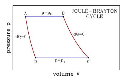
Figure 2.42: A Joule-Brayton cycle consists of two adiabats (dark red) and two isobars (light blue).
