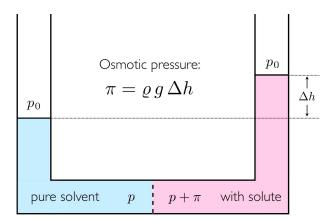
Figure 2.29: Osmotic pressure causes the column on the right side of the U-tube to rise higher than the column on the left by an amount  $\Delta h = \pi/\varrho g$ .
