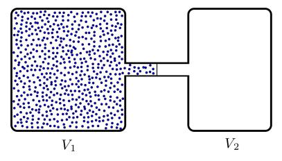
Figure 2.10: In the adiabatic free expansion of a gas, there is volume expansion with no work or heat exchange with the environment:  $\Delta E = Q = W = 0$ .
