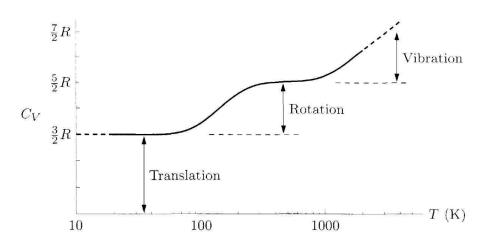
Figure 2.8: Heat capacity  $C_V$  for one mole of hydrogen (H<sub>2</sub>) gas. At the lowest temperatures, only translational degrees of freedom are relevant, and f = 3. At around 200 K, two rotational modes are excitable and f = 5. Above 1000 K, the vibrational excitations begin to contribute. Note the logarithmic temperature scale. (Data from H. W. Wooley *et al.*, Jour. Natl. Bureau of Standards, **41**, 379 (1948).)
