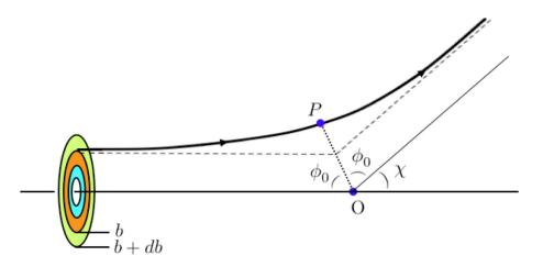
Figure 8.6: Scattering in the CM frame. O is the force center and P is the point of periapsis. The impact parameter is b, and  $\chi$  is the scattering angle.  $\phi_0$  is the angle through which the relative coordinate moves between periapsis and infinity.
