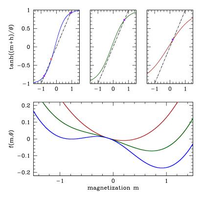
Figure 7.10:  $f(m,\theta,h)$  for h = 0.1. Upper panels: graphical solution to the self-consistency equation  $m = \tanh((m+h)/\theta)$  at temperatures  $\theta = 0.65$  (blue),  $\theta = 0.9$  (dark green), and  $\theta = 1.5$  (dark red). Lower panel: mean field free energy, with energy shifted by  $\theta \ln 2$  so that  $f(\theta, m = 0) = 0$ .
