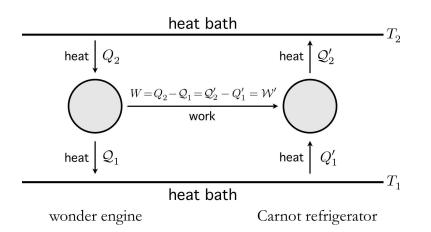
Figure 2.13: A wonder engine driving a Carnot refrigerator.
