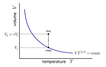
Figure 2.17: Adiabatic free expansion via a thermal path. The initial and final states do not lie along an adabat! Rather, for an ideal gas, the initial and final states lie along an isotherm.
