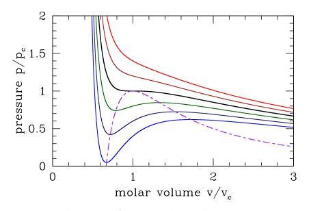
Figure 7.1: Pressure versus molar volume for the van der Waals gas at temperatures in equal intervals from  $T = 1.10 T_{\rm c}$  (red) to  $T = 0.85 T_{\rm c}$  (blue). The purple curve is  $\bar{p}^*(\bar{v})$ .
