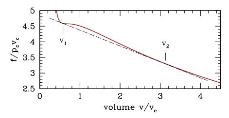
Figure 7.2: Molar free energy f(T, v) of the van der Waals system  $T = 0.85 T_c$ , with dot-dashed black line showing Maxwell construction connecting molar volumes  $v_{1,2}$  on opposite sides of the coexistence curve.
