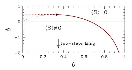
Figure 7.24: Mean field phase diagram for the Blume-Capel model. The black dot signifies a tricritical point, where the coefficients of  $m^2$  and  $m^4$  in the Landau free energy expansion both vanish. The dashed curve denotes a first order transition, and the solid curve a second order transition. The thin dotted line is the continuation of the  $\delta_{\rm c}(\theta)$  relation to zero temperature.
