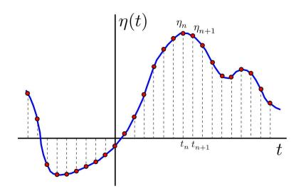
Figure 9.1: Discretization of a continuous function  $\eta(t)$ . Upon discretization, a functional  $\Phi[\eta(t)]$  becomes an ordinary multivariable function  $\Phi(\{\eta_i\})$ .
