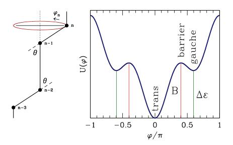
Figure 6.21: Left: trans and gauche orientations in carbon chains. Right: energy as a function of azimuthal angle  $\varphi$ . There are three low energy states: trans ( $\varphi = 0$ ) and gauche ( $\varphi = \pm \varphi_0$ ).
