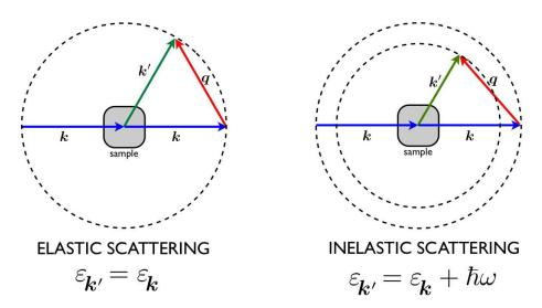
Figure 6.17: In a scattering experiment, a beam of particles interacts with a sample and the beam particles scatter off the sample particles. A momentum  $\hbar q$  and energy  $\hbar \omega$  are transferred to the beam particle during such a collision. If  $\omega = 0$ , the scattering is said to be *elastic*. For  $\omega \neq 0$ , the scattering is *inelastic*.
