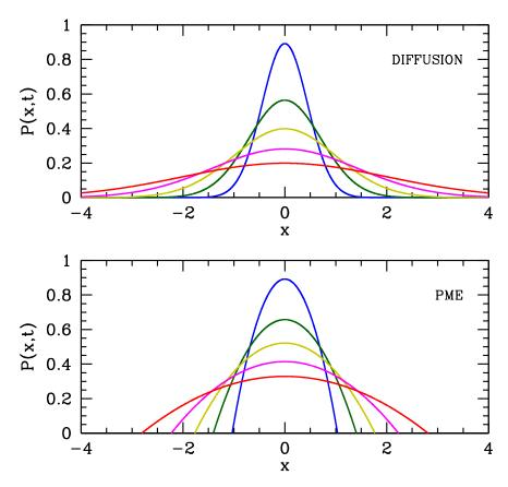
Figure 9.5: Top panel: evolution of the diffusion equation with D = 1 and  $\sigma = 1$  for times t = 0.1, 0.25, 0.5, 1.0, and 2.0. Bottom panel: evolution of the porous medium equation with m = 2 and d = 1 and C chosen so that P(x = 0, t = 0.1) is equal to the corresponding value in the top panel (*i.e.* the peak of the blue curve).
