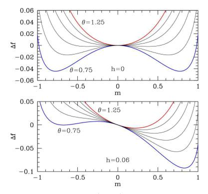
Figure 7.13: Variational field free energy  $\Delta f = f(m, h, \theta) + \theta \ln 2$  versus magnetization m at six equally spaced temperatures interpolating between 'high' ( $\theta = 1.25$ , red) and 'low' ( $\theta = 0.75$ , blue) values. Top panel: h = 0. Bottom panel: h = 0.06.
