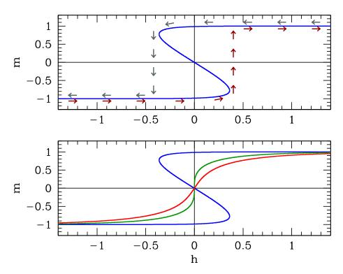
Figure 7.12: Top panel : hysteresis as a function of ramping the dimensionless magnetic field h at  $\theta = 0.40$ . Dark red arrows below the curve follow evolution of the magnetization on slow increase of h. Dark grey arrows above the curve follow evolution of the magnetization on slow decrease of h. Bottom panel : solution set for  $m(\theta, h)$  as a function of h at temperatures  $\theta = 0.40$  (blue),  $\theta = \theta_c = 1.0$  (dark green), and t = 1.25 (red).
