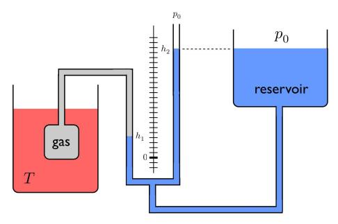
Figure 2.3: The constant volume gas thermometer. The gas is placed in thermal contact with an object of temperature T. An incompressible fluid of density  $\rho$  is used to measure the pressure difference  $\Delta p = p_{\text{gas}} - p_0$ .
