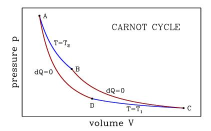
Figure 2.14: The Carnot cycle consists of two adiabats (dark red) and two isotherms (blue).
