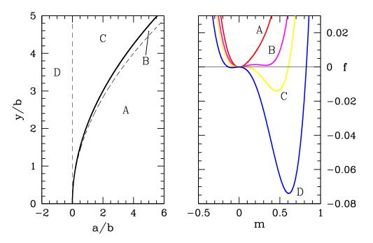
Figure 7.15: Behavior of the quartic free energy  $f(m) = \frac{1}{2}am^2 - \frac{1}{3}ym^3 + \frac{1}{4}bm^4$ . A:  $y^2 < 4ab$ ; B:  $4ab < y^2 < \frac{9}{2}ab$ ; C and D:  $y^2 > \frac{9}{2}ab$ . The thick black line denotes a line of first order transitions, where the order parameter is discontinuous across the transition.
