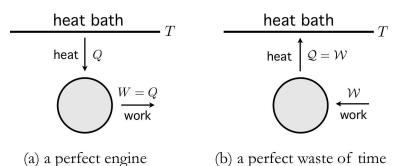
Figure 2.11: A *perfect engine* would extract heat Q from a thermal reservoir at some temperature T and convert it into useful mechanical work W. This process is also impossible, according to the Second Law of thermodynamics. The inverse process, where work W is converted into heat Q, is always possible.
