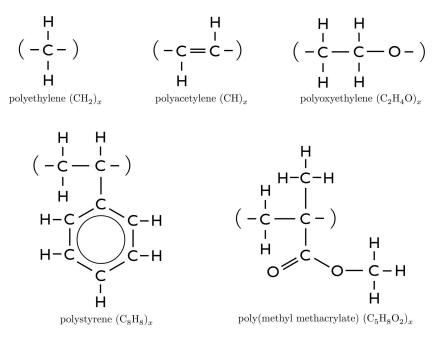
Figure 6.20: Some examples of linear chain polymers.
