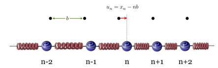
Figure 5.3: A linear chain of masses and springs. The black circles represent the equilibrium positions of the masses. The displacement of mass n relative to its equilibrium value is  $u_n$ .
