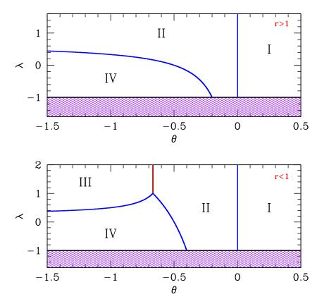
Figure 7.28: Phase diagram for  $\tau = 0.5$ , r = 1.5 (top) and  $\tau = 0.5$ , r = 0.25 (bottom). The hatched purple region is unphysical, with a free energy unbounded from below. The blue lines denote second order transitions. The thick red line separating phases II and III is a first order line.
