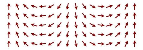
Figure 7.22: A domain wall in an XY ferromagnet.
