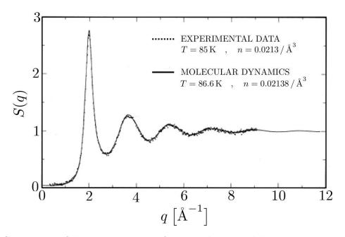
Figure 6.18: Comparison of the static structure factor as determined by neutron scattering work of J. L. Yarnell *et al.*, *Phys. Rev. A* **7**, 2130 (1973) with molecular dynamics calculations by Verlet (1967) for a Lennard-Jones fluid.
