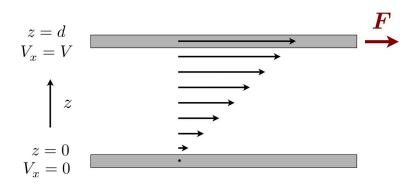
Figure 8.4: Gedankenexperiment to measure shear viscosity  $\eta$  in a fluid. The lower plate is fixed. The viscous drag force per unit area on the upper plate is  $F_{\text{drag}}/A = -\eta V/d$ . This must be balanced by an applied force F.
