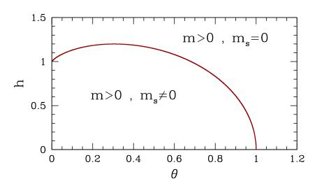
Figure 7.26: Mean field phase diagram for the Ising antiferromagnet in an external field. The phase diagram is symmetric under reflection in the h = 0 axis.
