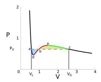
Figure 7.4: Maxwell construction in the (v, p) plane. The system is absolutely unstable between volumes  $v_{\rm d}$  and  $v_{\rm e}$ . For  $v \in [v_{\rm a}, v_{\rm d}]$  of  $v \in [v_{\rm e}, v_{\rm c}]$ , the solution is unstable with respect to phase separation. Source: Wikipedia.
