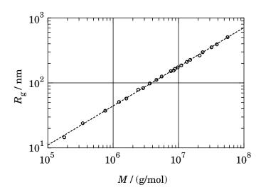
Figure 6.23: Radius of gyration  $R_{\rm g}$  of polystyrene in a toluene and benzene solvent, plotted as a function of molecular weight of the polystyrene. The best fit corresponds to a power law  $R_{\rm g} \propto M^{\nu}$  with  $\nu = 0.5936$ . From J. Des Cloizeaux and G. Jannink, *Polymers in Solution: Their Modeling and Structure* (Oxford, 1990).
