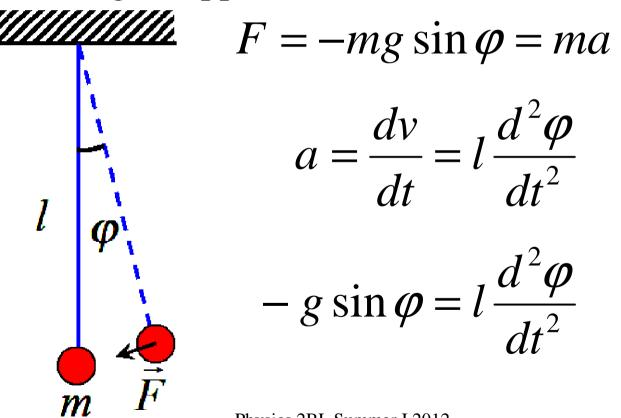
Measure g with simple pendulum Don't know how to solve EOM:  $-g \sin \varphi = l \frac{d^2 \varphi}{dt^2}$ Simplify with small angle approx:  $\sin \varphi \approx \varphi$ EOM simplifies
