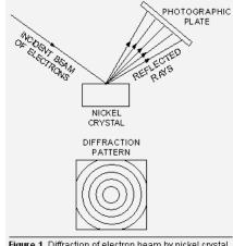
Figure 1. Diffraction of electron beam by nickel crystal (Davisson and Germer's experiment)
