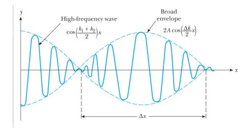
□ Group velocity: speed of the blue envelope □ Blue:  $v_g = \Delta \omega / \Delta k$ , just like Red:  $v_p = \omega / k$
