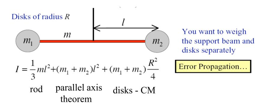
$$\sigma_{I} = \begin{bmatrix} (\delta I / \delta m) \sigma_{m} ]^{2} + [(\delta I / \delta m_{1}) \sigma_{m1} ]^{2} + \\ [(\delta I / \delta m_{2}) \sigma_{m2} ]^{2} + [(\delta I / \delta l) \sigma_{l} ]^{2} + [(\delta I / \delta R) \sigma_{r} ]^{2} \end{bmatrix}$$
