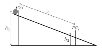
a ramp. The ball will start from rest at a height,  $h_1$ , at the first photogate,  $PG_1$ . We will measure the time, t, that it takes for the ball to get to travel a distance, x, when it arrives at a second photogate,  $PG_2$ , which is at a height,  $h_2$ . As long as the ball starts at rest, the change in potential energy due to the change in height,  $h = h_1 - h_2$ , is converted into a final rotational and a final translational kinetic energy.
