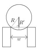
In our experiment there is a slight complication because the ball is not rolling on a flat surface but rather a square beam that is open on the top (See a cross of the ball sitting in this beam on page 1). This means that the rolling radius of the ball is smaller than its actual radius. We can calculate the rolling radius, R', by measuring the width of the beam and using the Pythagorean Theorem,
