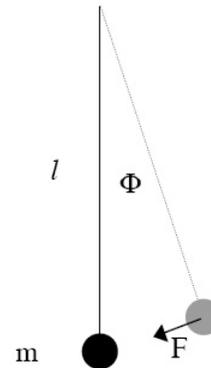
In order to measure  $g$  a simple pendulum will be constructed which will consist of a mass hanging from string. For this derivation a dot means first derivative in time and a double dot means second derivative in time. Initially the mass is displaced a small angle,  $\phi(t=0) = \phi_0$ , with no initial angular velocity,  $\dot{\phi}(t=0) = 0$ . A small component of the force of gravity torques the mass towards the equilibrium point. Using the small angle approximation (See Appendix 1):
