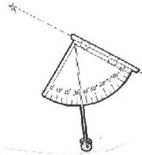
This is a simple version of a sextant, an instrument used to measure angles in comparison to a plumb vertical line.
