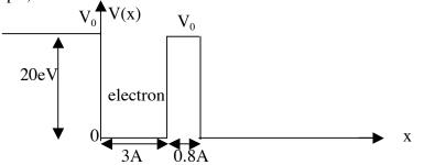
An electron is in the potential well shown in the figure, of depth  $V_0=20eV$  and width 3A. (a) Find the energy of the ground state and the first excited state. You may assume it is an infinite well and get approximate answers. State whether the exact answers will be larger or smaller than the approximate answer, and for which of the two states (ground state or first excited state) is the error larger and why.
