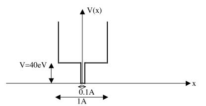
A particle moves in the one-dimensional potential well V(x) shown in the figure. The potential is V= $\infty$  for |x|>0.5A, V=40eV for 0.05A<|x|<0.5A and V=0 for -0.05A<x<0.05A. It is difficult to solve the Schrodinger equation exactly for this potential, but you should be able to give approximate answers to the following questions.
