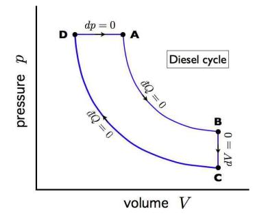
Figure 2: A Diesel cycle consists of two adiabats, an isobar, and an isochore.
