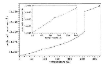
Figure 1: Temperature variation of the cubic lattice constant a(T) of  $C_{60}$  as a function of temperature, from W. I. F. David *et al.*, *Europhys. Lett.* **18**, 219 (1992).
