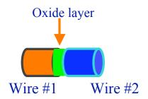
Q: 2 Cu wires are seperated by insulating Oxide layer. Modeling the Oxide layer as a square barrier of height U=10.0eV, estimate the transmission coeff for an incident beam of electrons of E=7.0 eV when the layer thickness is (a) 5.0 nm (b) 1.0nm
