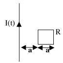
The figure shows a straight vertical long wire carrying a time-dependent current  $I(t)=I_0\ t^2/\tau^2$ , with  $I_0=100A$  and  $\tau=1s$ . The square loop shown has resistance  $R=1\Omega$  and sides of length a=25cm. Two sides of the square loop are parallel to the long wire, with the closest one at distance a from the long wire.
