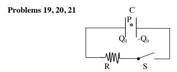
In the circuit shown, the parallel plate capacitor has capacitance 3mF and has round plates of radius a=0.4m. The resistor has resistance  $250\Omega$ . Initially the charge on the capacitor is  $Q_0=5C$ , with the left capacitor plate having positive charge, and the switch S is open. At time t=0 the switch S is closed.
