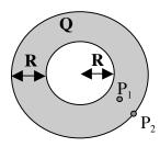
The figure shows a non-conducting spherical shell of inner radius R and outer radius 2R (i.e. radial thickness R) with charge Q uniformly distributed throughout its volume.
