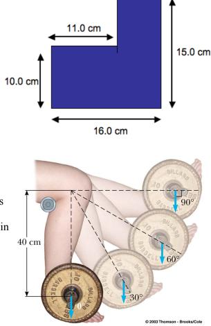
**3.** As part of a physical therapy program following a knee operation, a 5.0 kg object is attached to an ankle and leg lifts are done as sketched in the figure. Calculate the torque (in units of N-m) about the knee due to this weight for the four positions shown.
