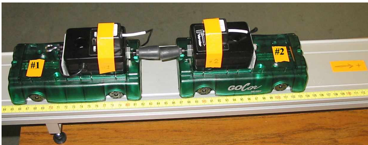
Carts 1 and 2 with force sensors and accelerometers. Positive direction is \rightarrow
