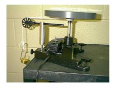
We will be focusing on the hanging mass for the measured values of this experiment. The hanging mass would fall at a rate of  $9.8 \text{ m/s}^2$  except that it has a tension force due to the string that is slowing it down. Our goal is to find the acceleration value of the hanging mass,  $a_y$ , by measuring the time it takes for the mass to fall a given value,  $\Delta y$ .
